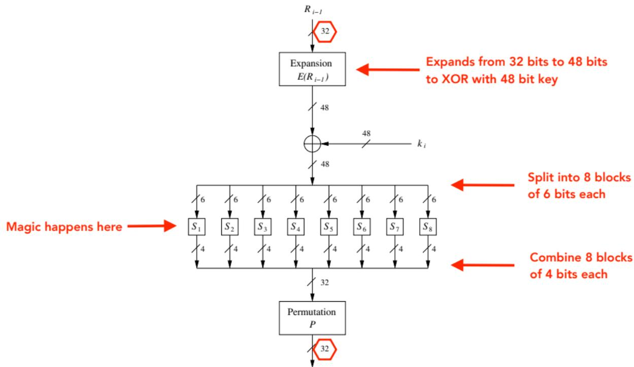
**Fig. 3.10** Block diagram of the  $f$ -function
